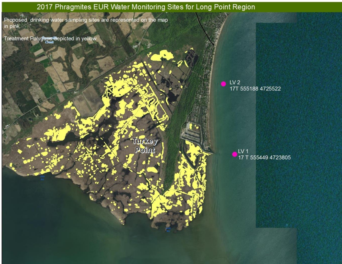
Figure 1: Two proposed water sample locations to cover off the Turkey Point area. LV1 as the main sample site and LV2 (water intake location) as an alternate should glyphosate levels meet or exceed 0.028mg/L.
